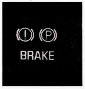
Your vehicle's hydraulic brake system is divided into two parts. If one part isn't working, the other part can still work and stop you. For good braking, though, you need both parts working well.
